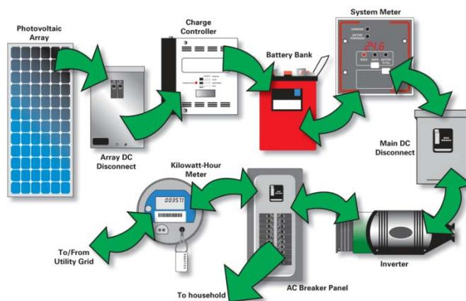
Figure 1. Typical Grid-Connected PV System<sup>23</sup>
